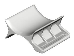
Clamp clips allows both cables and pipes to be fastened to profile rails. The clamp clips are hooked into the appropriate slot widths of the profile rails and the component to be fastened is pressed onto the profile rail with the pressure trough of the clamp clip and held in place.
