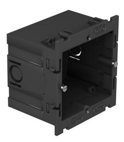
Accessory mounting box to accept standard switching and connection devices in support ring and support clamp versions of all manufacturers. An extra-large installation opening means that the box is particularly suited to accept ELKO devices as well as larger versions of data technology connection sockets. The protective housing is not essential for data technology applications.
