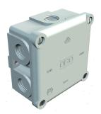
Protection rating IP54, rated voltage 660 V, nominal cross-section 2.5  $\div$  4, in combination with the earthing terminal 700/6 M, the box has the nominal crosssection 4 mm², two fastening holes for screws of up to 5 mm  $\varnothing$  on the outer side of the box. Four cover screws, 7 break-out entries with thread M20 x 1.5, primarily for cable glands with short connecting thread.
