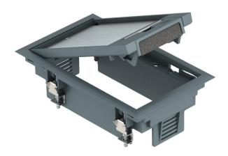
Service outlet with handle clamp for up to 3 individual Modul 45 devices in one UT3 universal support, use in duct systems and system floors for indoor use. Up to two installation devices with 50 mm central plate can be inserted. Service outlet with handle clamp, 1-compartment, for the installation of MT2 mounting support.
