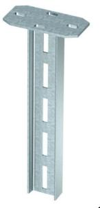
I support with welded head plate. For fastening to horizontal concrete ceilings and steel girders. Single and double-sided brackets of type AS 15, AS 30 and AS 55 can be fastened to the IS 8 K suspended support. The height of the brackets is infinitely adjustable.
