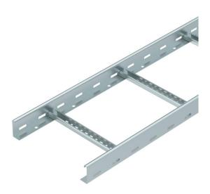
Cable ladder with perforated side rail of side height 60 mm with riveted C profile frames, open in an upwards direction (VS version). The cable ladder is shipped folded up.
