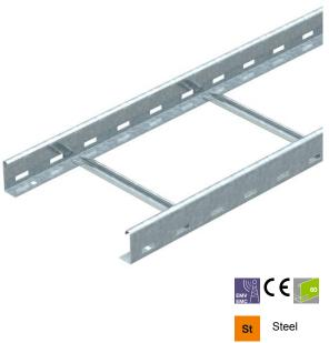
Cable ladder with perforated side rail of side height 60 mm with riveted C profile rungs, open in an upwards direction (NS version).
