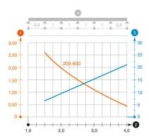
Load diagram, cable ladder, type LG 60 NS
