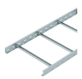
Cable ladder with perforated side rail of side height 60 mm with riveted C profile frames, open in an upwards direction (VS version). The cable ladder is shipped folded up.
