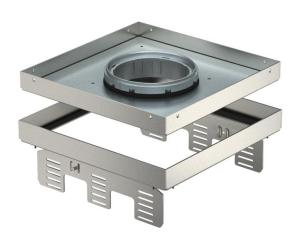
Height-adjustable cassette, decoupled from the floor, of nominal size 9, for tube bodies, for the installation of accessories in dry or wet-cleaned floors for indoor use, for mounting in underfloor boxes UZD250-3 or UZD350-3, either in conjunction with a mounting lid DUG. //9 or in UGD250-3/9 or UGD350-3/9. Mounting takes place using height adjustment brackets (order separately) in the aluminium frame profile of the underfloor boxes.
