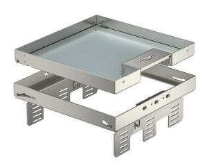
Height-adjustable cassette, decoupled from the floor, of nominal size 9, with cord outlet, for the installation of accessories in dry-cleaned floors indoors, for mounting in underfloor boxes UZD250-3 or UZD350-3, either in conjunction with a mounting cover DUG../9 or in UGD250-3/9 or UGD350-3/9. Mounting takes place using height-adjustment brackets (order separately) in the aluminium frame profile of the underfloor boxes.
