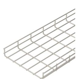
Mesh cable tray made of spot-welded steel wire of side height 55 mm. The grid width is 50 x 100 mm. Magnetic shield insulation without cover 15 dB, with cover 25 dB.
