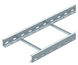
Cable ladder with 60 mm side height with riveted C profile rungs which are open in an upwards direction. Rolled side rail for reinforcement and as edge protection. Fastening to the bracket takes place using clamp, type LKS 40. The slot dimension of the frame is 11 mm and the appropriate U clamp is type 2056/N. Magnetic shield insulation without cover 10 dB, with cover 15 dB.
