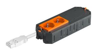
The ready-for-connection UTC4 universal support has 2 pre-installed 33° protective contact sockets of 16 A and 2 blanking covers for retroinstallation of 2 installation devices of the Modul 45 series. Suitable for VL connection cables and device installation units of nominal size R7, R9 and 9.
