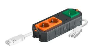
The ready-for-connection UTC4 universal support has 2 pre-installed 33° protective contact sockets in orange and one pre-installed 33° protective contact socket in mint green and one blanking cover for retroinstallation of an installation device of the Modul 45 or Modul 45connect series, 250 V~, 16 A.
