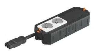
The ready-for-connection UTC4 universal support has 2 pre-installed 33° protective contact sockets in white and 2 blanking covers for retroinstallation of 2 installation devices of the Modul 45 series. Suitable for VL connection cables and device installation units of nominal size R7, R9 and 9.
