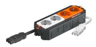
The ready-for-connection UTC4 universal support possesses 2 pre-installed  $33^\circ$  protective contact sockets in white and 2 pre-installed  $33^\circ$  protective contact sockets in orange (with surge protection module, type 3, according to DIN EN 61643-11), 250 V~, 16 A. Suitable for VL connection cables and device installation units of nominal size R7, R9 and 9.
