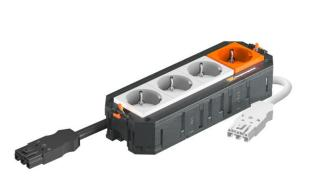
The ready-for-connection UTC4 universal support possesses 3 pre-installed 33° protective contact sockets in white and 1 pre-installed 33° protective contact socket in orange (with surge protection module, type 3, according to DIN EN 61643-11), 250 V~, 16 A. Suitable for VL connection cables and device installation units of nominal size R7, R9 and 9.
