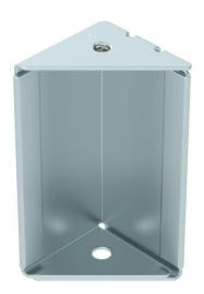
Additional support for the elevation of the walkable BKRS cable tray system on the floor. Required for elevations with Z supports ZST from a tray width of 500 mm. Fastening with flat head screw FKS 6x12 mm (item no. 6049246).
